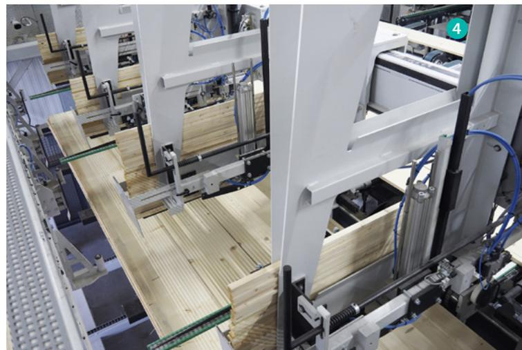
going along the bypass, it passes the planing machine and enters the packaging unit directly. "This way, the plant can be used very flexibly, even just for rip-cutting with the Profisplit," Weinig representative Peter Haas explains.
